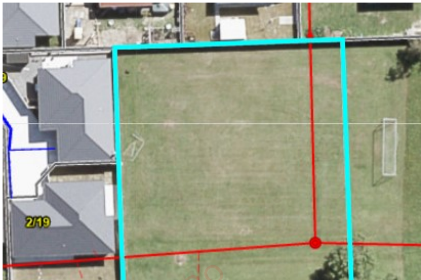
Figure 3: Wastewater main traversing the northern rear of the application site.
