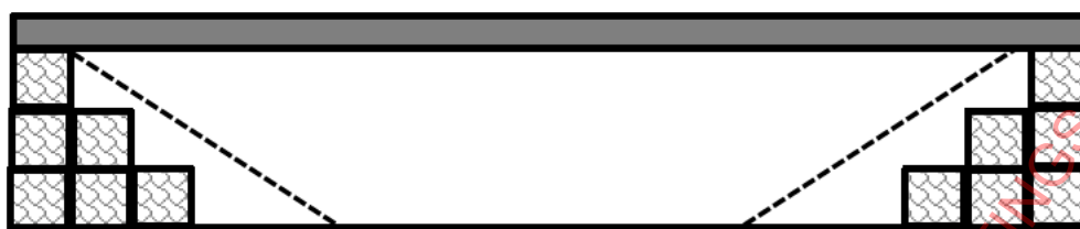
Figure 7-14 Sketch of proposed cross section widening under Nelson Crescent Bridge
