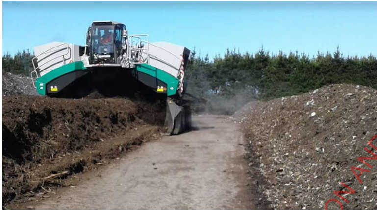
Photograph Appendix C.6: Open Windrow Composting with a specialist windrow turner.
