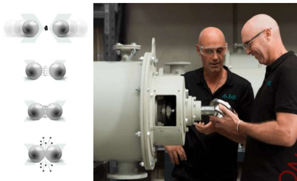
Figure 2: Utilising the mechanical energy of high-velocity ball bearings within specialised reactors
