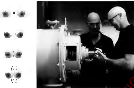
Figure 2: Utilising the mechanical energy of high-velocity ball bearings within specialised reactors
