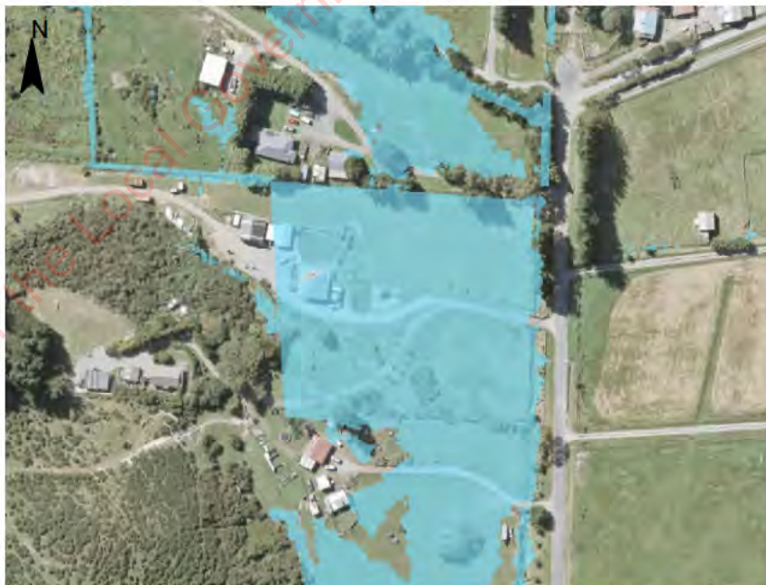
Figure 7-4 Storage C at Upper Fitzherbert (1% AEP + 20% CC storm event) (location indicative only)
