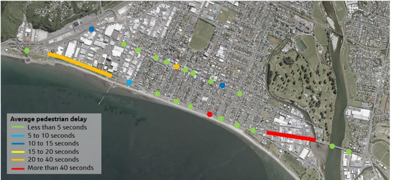
Figure 16 Pedestrian Delays in the Study Area
